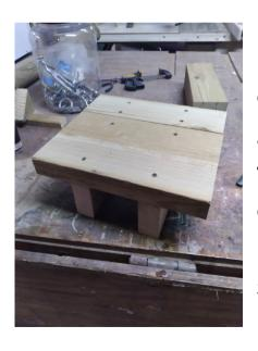
b) Lay parts 1 and 1 b on top of parts 2 and 2 b and screw together using 3½" deck screws, then remove the 4x4 spacer.
